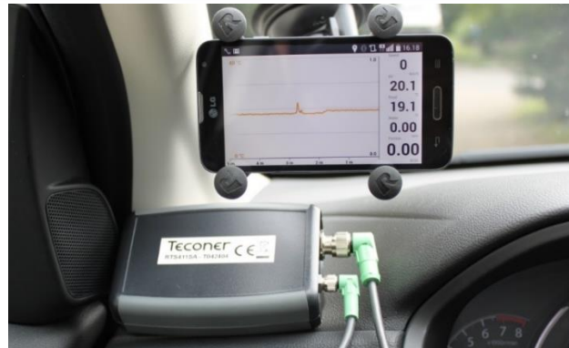
Photograph of the user interface with temperature measurements and the Bluetooth communication enclosure inside the vehicle.
