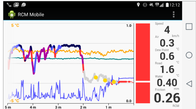
Screenshot of the mobile device user interface with temperature and road condition measurements.
